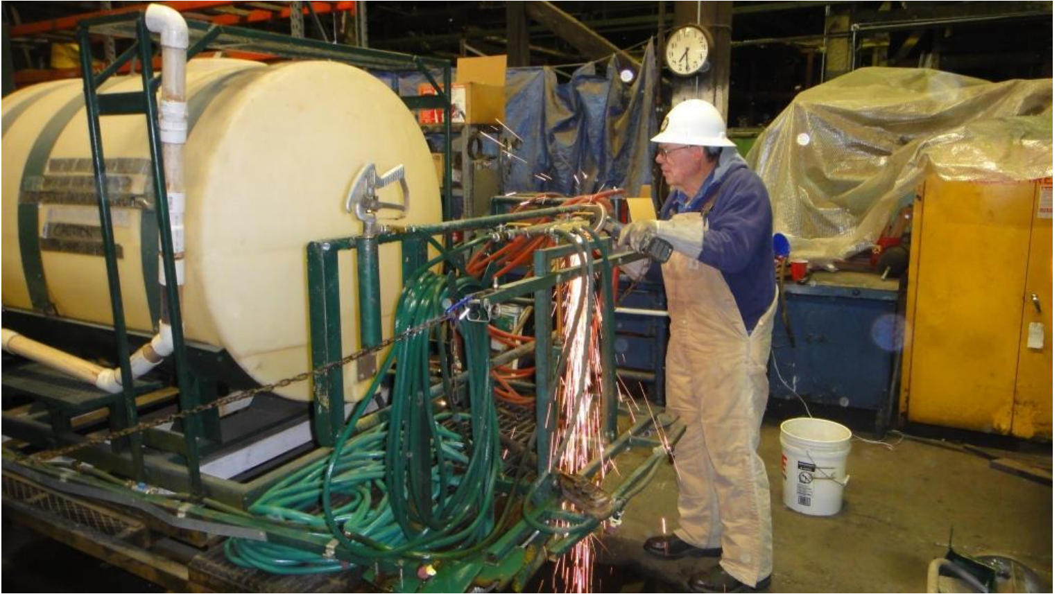
Cliff making modifications to the Weed Team's 500-gallon spray-rig getting it ready for the 2016 season
